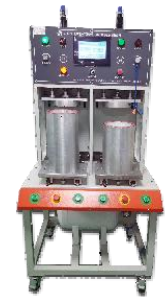
Airtightness tester (6 sets)
