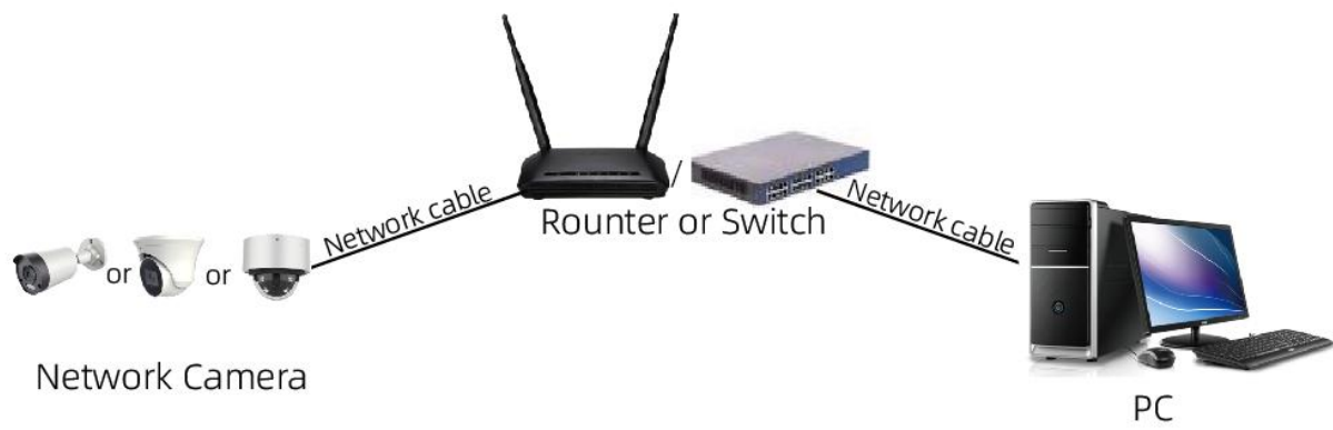
Figure 1-2 Connecting via a Switch or a Router
